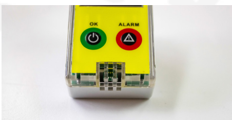
Internal humidity & temperature sensor in transducer's case
