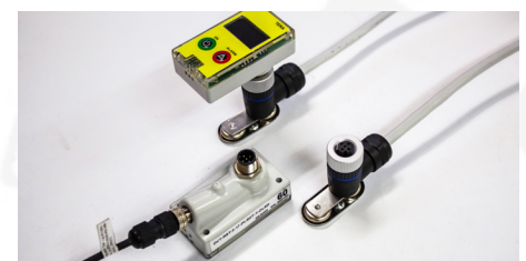
M12 connector for quick RS485 connection with a transducer
