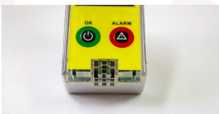
Internal humidity & temperature sensor in transducer's case
